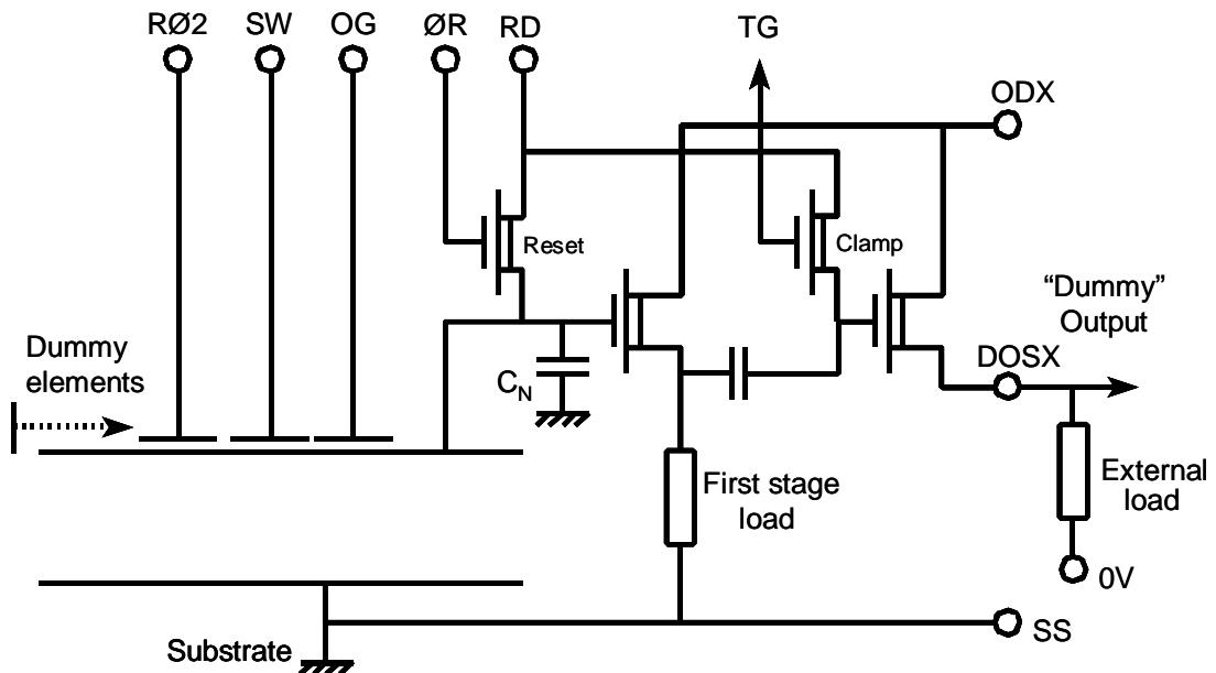
The first stage load of each output (real or dummy) draws a quiescent current of approximately 0.2 mA via SS.
