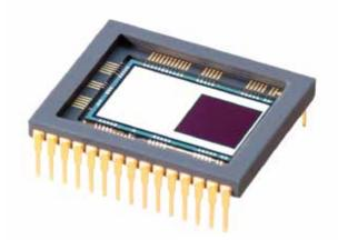
the area defined by one of the pixels will be converted into one (or more) electrons and the number of electrons collected will be directly proportional to the intensity of the scene at each pixel. When the CCD is clocked out, the number of electrons in each pixel are measured and the scene can be reconstructed.
