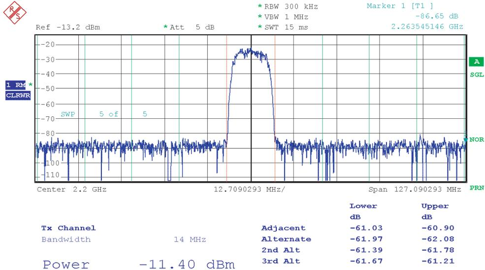
ACPR is in excess of 60 dB. DMWS capability is proven for the second Nyquist zone in RF mode with slightly reduced dynamic range regarding NRTZ mode but with increased output power.
