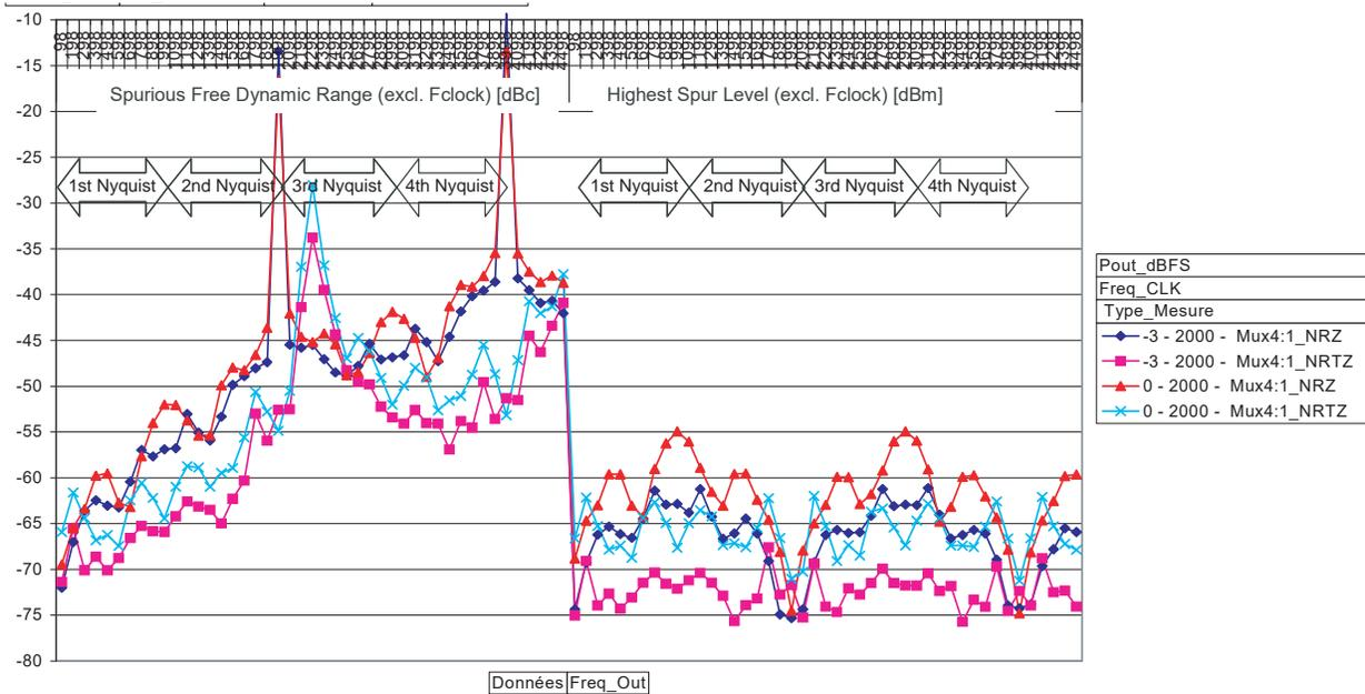
NRTZ linearity is slightly improved reducing the sampling rate to 2000 MSps, possibility of operation over the 4<sup>th</sup> Nyquist zone is demonstrated.
