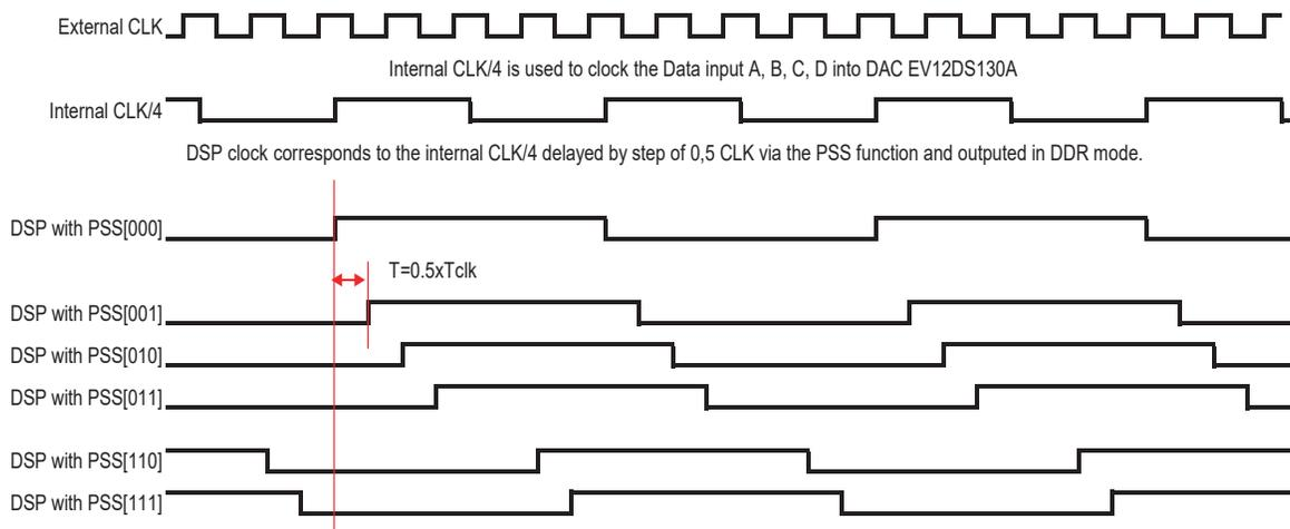
**Figure 5-9.** PSS Timing Diagram for 2:1 MUX, OCDS[00]
