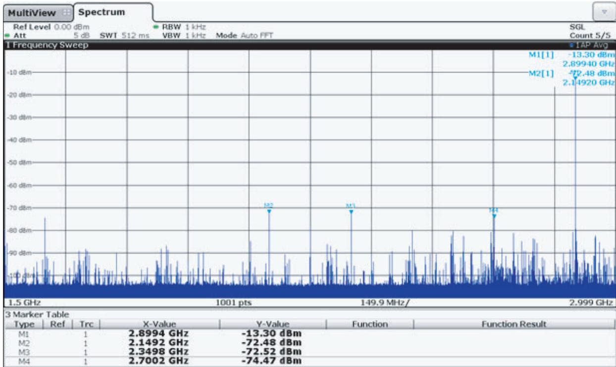
**Figure 7-24.** Typical SFDR spectrum in RF mode.  $F_{out} = 4400\text{MHz}$  (3rd Nyquist), MUX4:1,  $F_s = 3\text{Gps}$ . SFDR = 56 dBc
