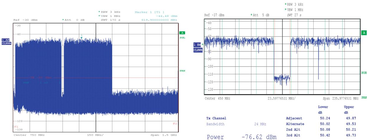
Measured average NPR: 50.02 dB, therefore SNR = 61.02 dB and ENOB = 9.84 bit
