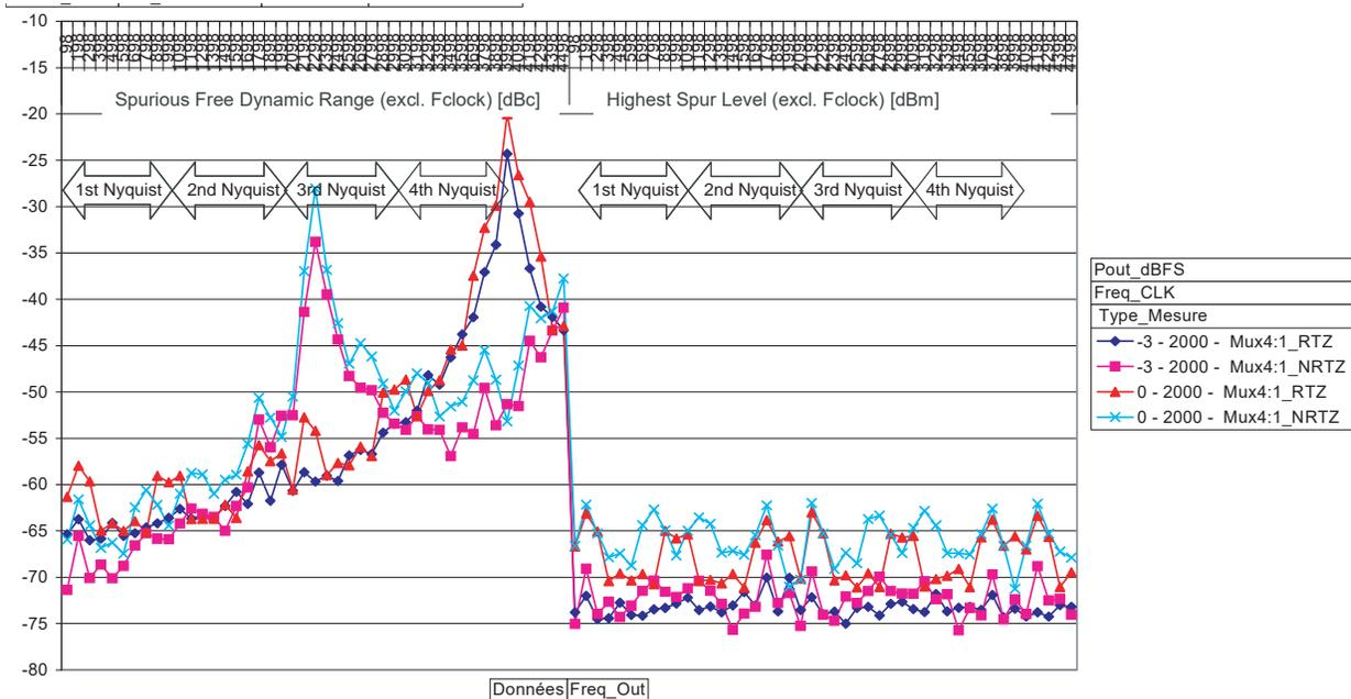
NRTZ mode is relevant in 1<sup>st</sup>, 2<sup>nd</sup> Nyquist zones and is still usable over 4<sup>th</sup> Nyquist zone with SFDR in excess of 50 dBc.
