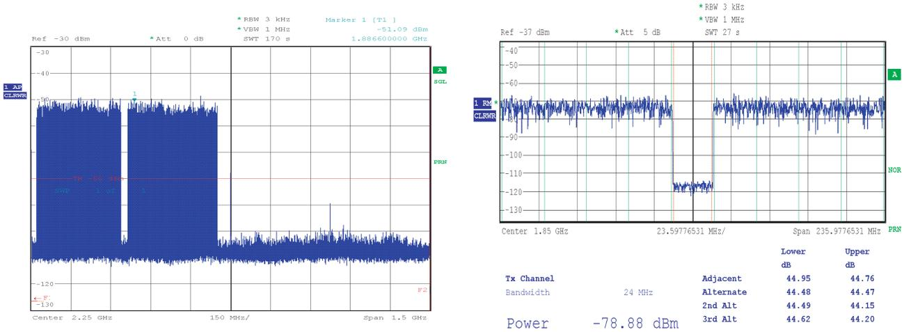
**Figure 7-45.** NPR in second Nyquist Zone, 1520 MHz to 2200 MHz noise pattern with a 25 MHz notch centered on 1850 MHz, RF Mode
