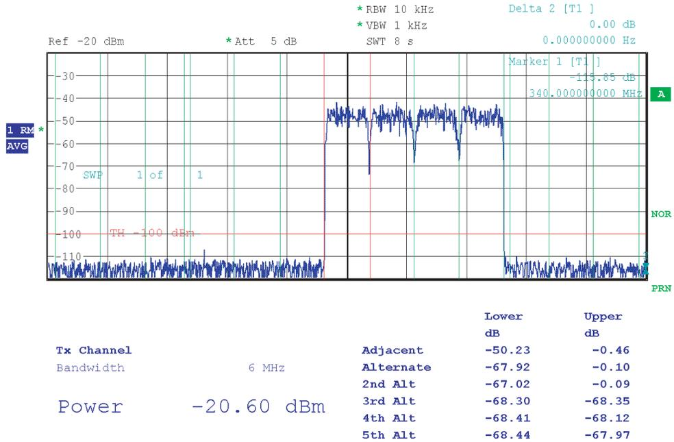
Figure 7-39. ACPR 1 Channel Centered on 900 MHz, Output Mode NRTZ
