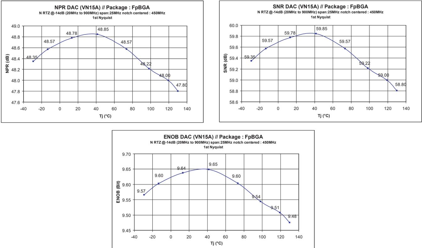
Optimum is at  $T_j = 40^{\circ}\text{C}$ , degradation over temp is within 1 dB (or 0.15 effective bit).
