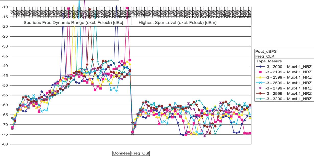
NRZ mode is only relevant for Fout below 400 MHz.
