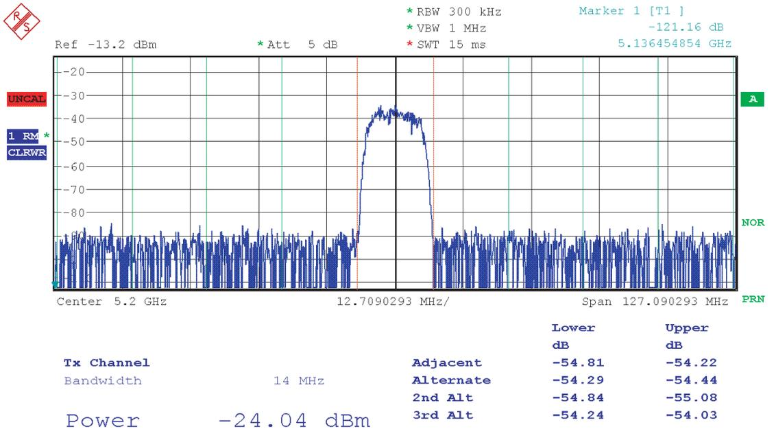
ACPR is in excess of 54 dB. DMWS capability is proven for the fourth Nyquist zone in NRTZ mode.
