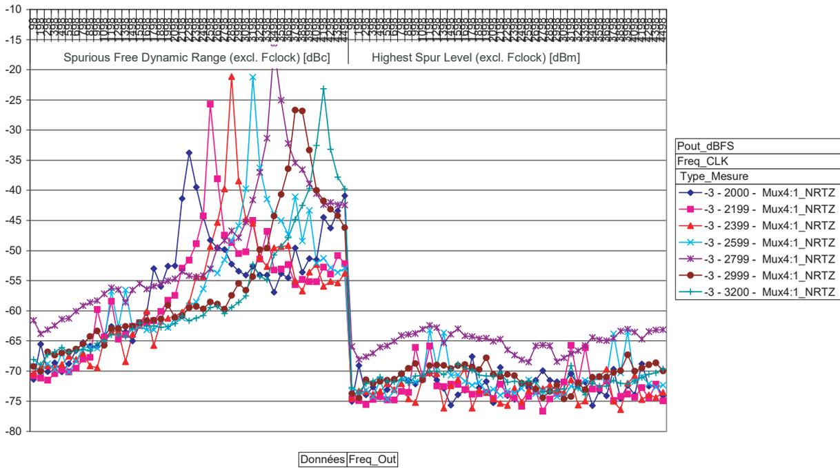
NRTZ mode brings significant improvement regarding NRZ mode. This mode concentrates the benefits of both NRZ mode (high power available) and RTZ mode (extended available dynamic range). The spikes in the SFDR are caused by normalization artefacts due to the Sinc(x) null.
