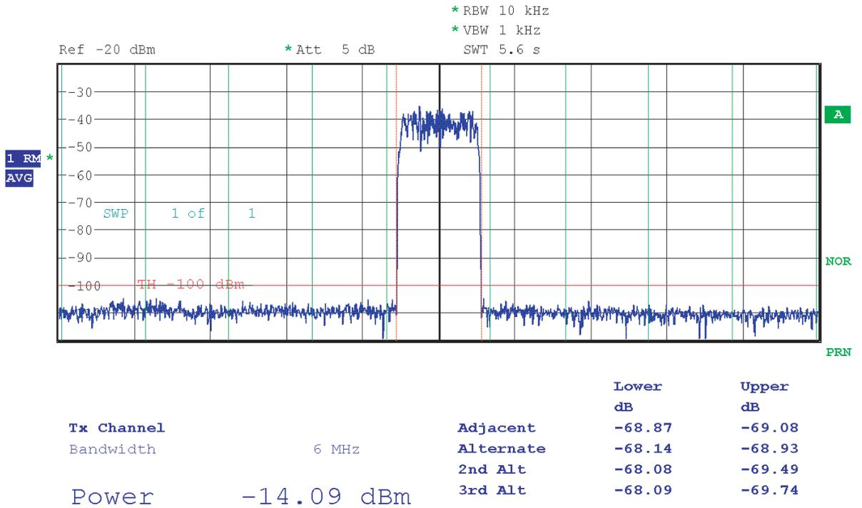
Figure 7-37. ACPR 1 channel centered on 300 MHz, Output Mode NRTZ
