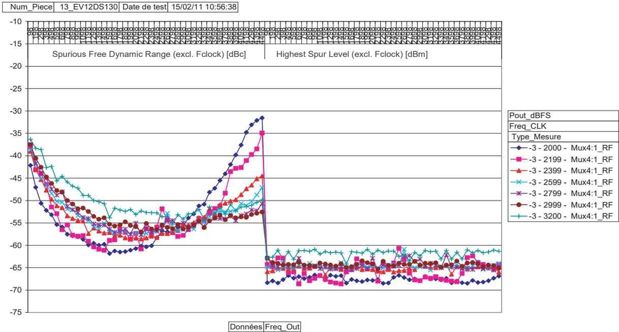
RF mode allows for operation over 3<sup>rd</sup> Nyquist zones. Performances are not sensitive to output level. Performance roll off occurs beyond 3000 MSps.
