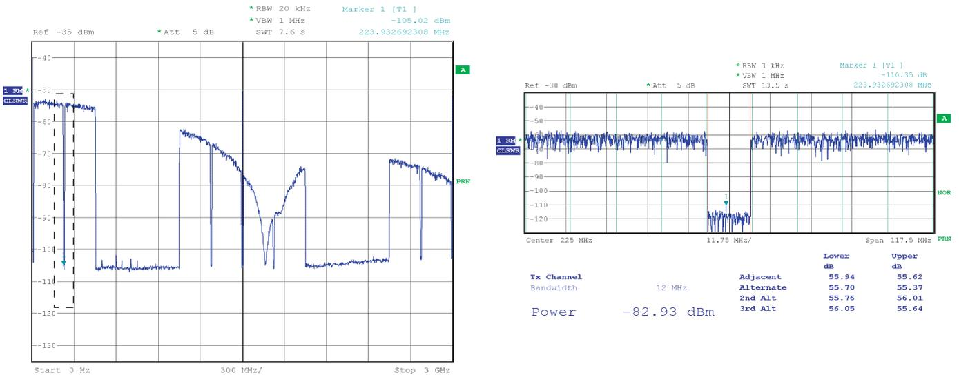
Measured average NPR: 55.7 dB, therefore SNR = 66.7 dB and ENOB = 10.8 bit.
