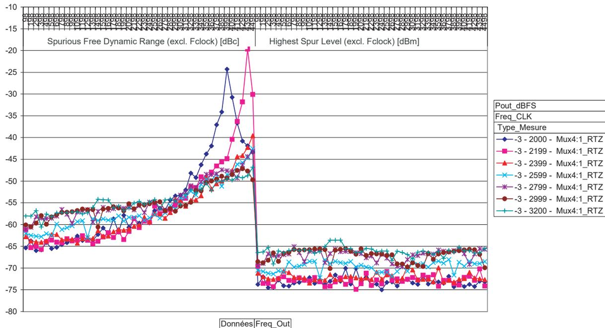
RTZ mode allows for operation over the 3 first Nyquist zones. In first and beginning of second Nyquist zone NRTZ mode is mode relevant. The spikes in the SFDR are caused by normalization artefacts due to the Sinc(x) null.
