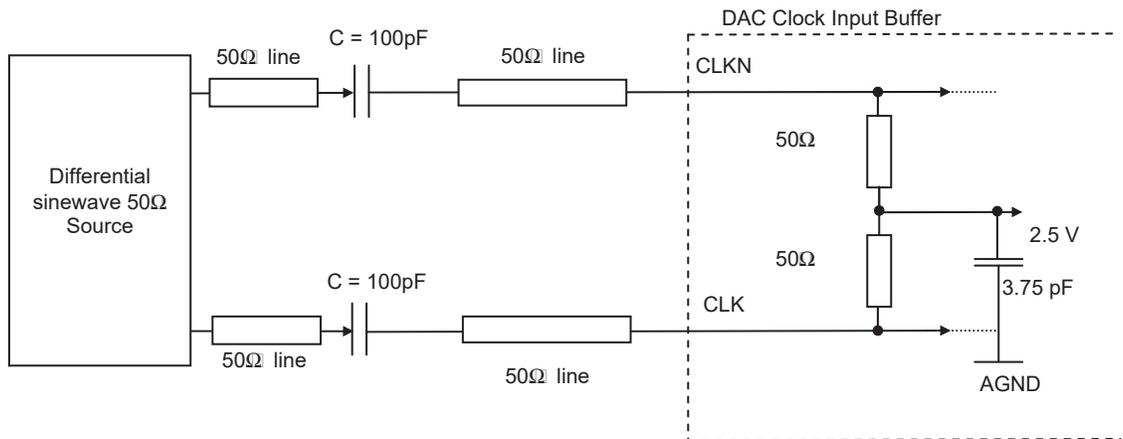
Note: The buffer is internally pre-polarized to 2.5V (buffer between  $V_{CC5}$  and AGND).
