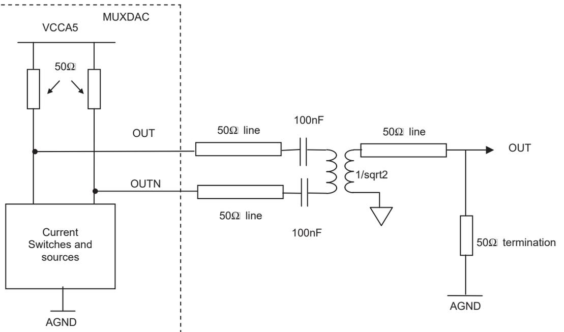
Note: The AC coupling capacitors should be chosen as broadband capacitors with a value depending on the application.
