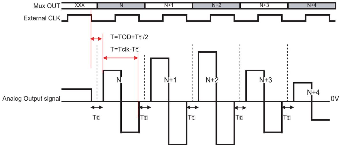
Note: The central transition is not hazardous but its elimination allows to push clock spur to  $2 \cdot F_s$
