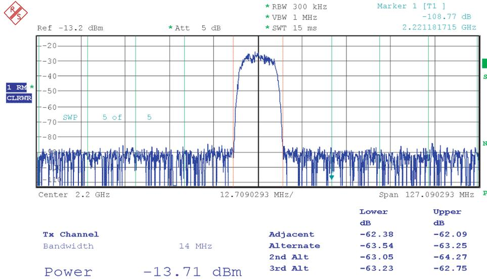
ACPR is in excess of 62 dB. DMWS capability is proven for second Nyquist in NRTZ mode.
