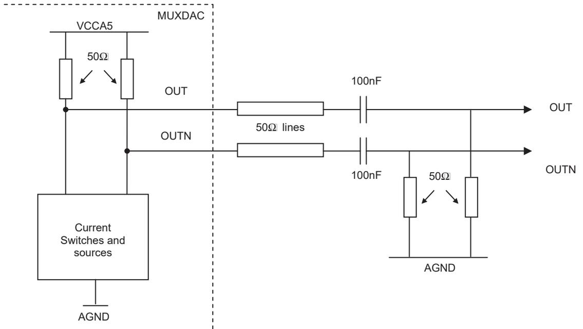
Figure 8-2. Analog Output Using a  $1/\sqrt{2}$  Balun
