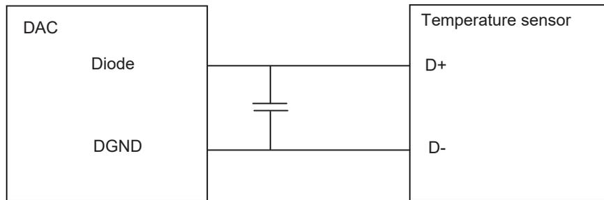
In characterization measurement a current of 1 mA is applied on the DIODE pin. The voltage across the DIODE pin and the DGND pin gives the junction temperature using the intrinsic diode characteristics below [Figure 5-17](#).
