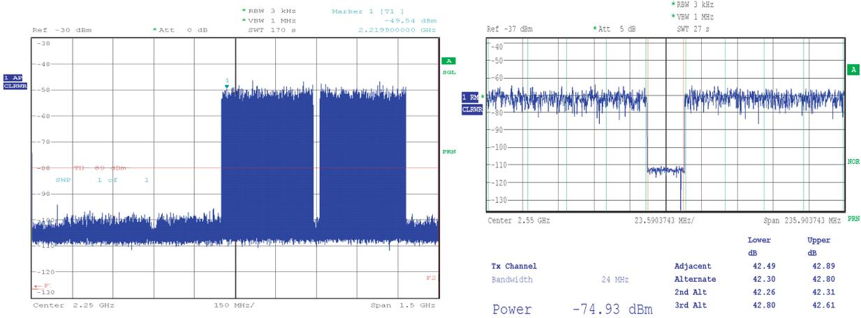
Measured average NPR: 42.56 dB, therefore SNR = 53.56 dB and ENOB = 8.6 bit.
