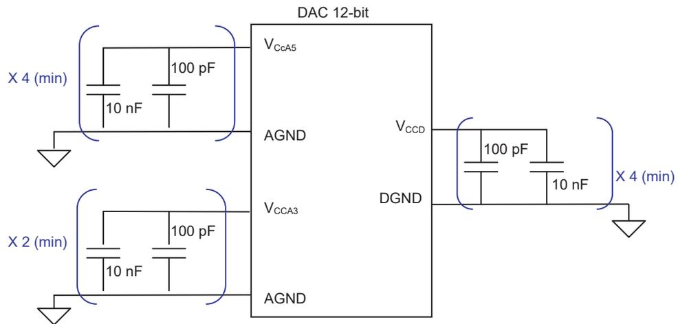
Each power supply has to be bypassed as close as possible to its source or access by 100 nF in parallel to 22  $\mu$ F capacitors (value depending of DC/DC regulators).
