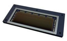
guarantee exceptional images with very high MTF. With  $5\mu m \times 5\mu m$  (PAN) and  $10\mu m \times 10\mu m$  (MS1-MS6) pixels these sensors provide extraordinary spatial resolution capability. The four Panchromatic bands have half pixel (2.5 $\mu$ m) offsets in both horizontal and vertical directions, allowing for super-resolution imaging to further enhance the resolution.
