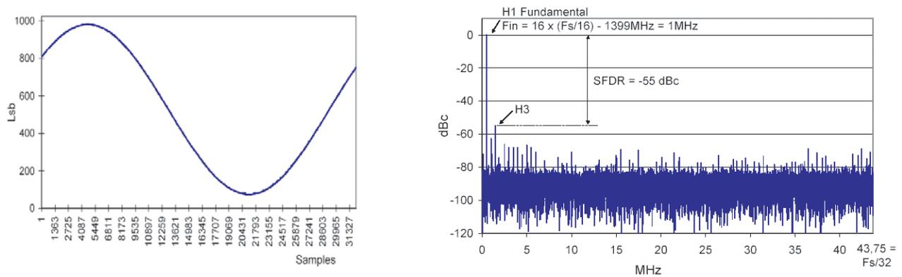
Figure 10-15.  $F_s = 1.7$  Gps and  $F_{in} = 898$  MHz, -1 dBFS; Decimation Factor = 16, 32 kpoints FFT
