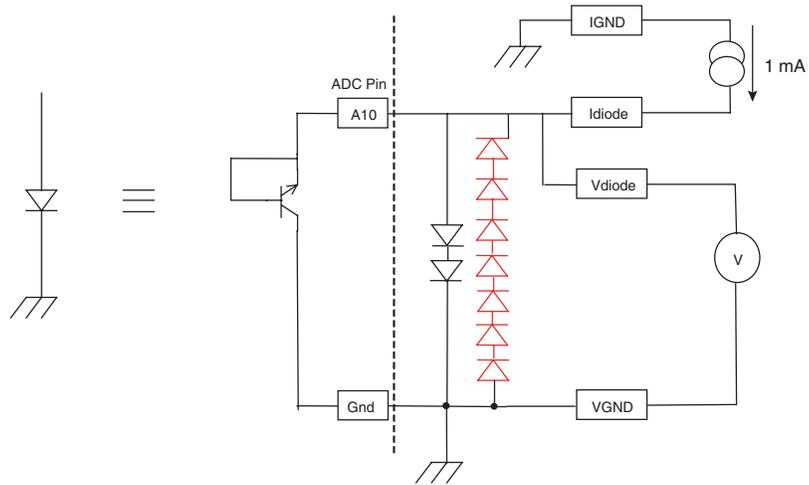
**Figure 13-13.** Diode Pin Implementation for Decimation Activation
