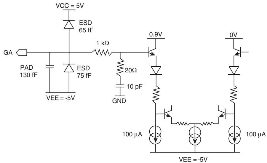
Figure 11-5. B/GB and PGEB Equivalent Input Schematics and ESD Protections
