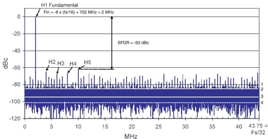
This is a 16384 points FFT. It is 16 times decimated since a DEMUX 1:8 is used to relax the acquisition system data rate, and data is captured on the rising edge of the data ready signal.
