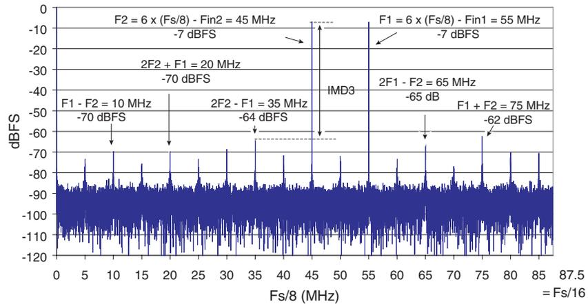
Note: The ADC input signal is sampled at 1.4 Gsps but the data acquisition is 8 times decimated. Thus, the spectrum is displayed from DC to  $F_s/2$  divided by the decimation factor  $[(F_s/2)/8 = 87.5 \text{ MHz}]$ .
