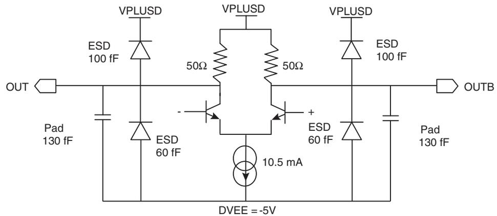
Figure 11-4. ADC Gain Adjust Equivalent Input Circuits and Protections
