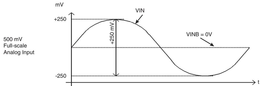
The analog full-scale input range is 0.5V peak-to-peak ( $V_{pp}$ ), or -2 dBm into the 50 Ω (100 Ω differential) termination resistor.
