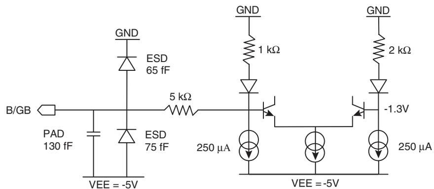
Figure 11-6. DRRB Equivalent Input Schematics and ESD Protections
