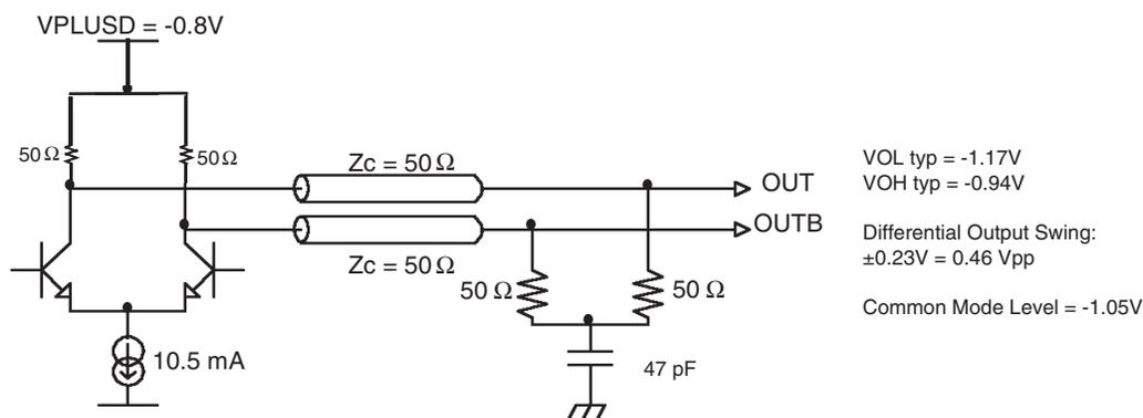
**Figure 13-8.** Unterminated Differential Outputs (Optional)
