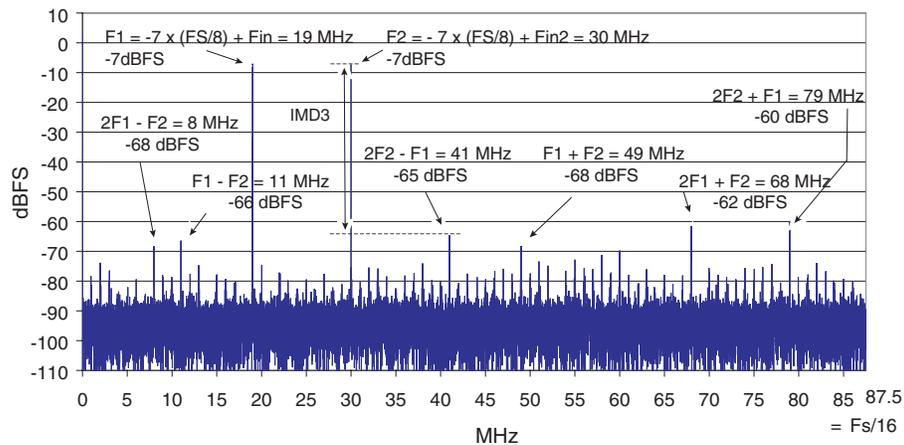
Note: The ADC input signal is sampled at 1.4 Gsps but data acquisition is 8 times decimated. Thus, the spectrum is displayed from DC to  $F_s/2$  divided by the decimation factor  $[(F_s/2)/8 = 87.5 \text{ MHz}]$ . The dual tone  $\text{IMD3}$  at 1.4 Gsps is around -65 dBFS for  $F_{in} = 1 \text{ GHz} \pm 250 \text{ MHz}$  ( $F_{in}$  range is from 750 MHz to 1250 MHz).
