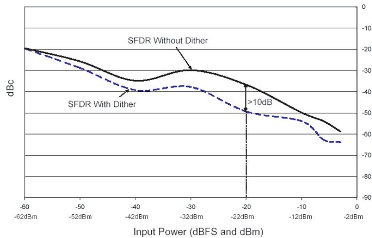
An increase in SFDR up to >10 dB with an addition of -23 dB<sub>rms</sub> DC to 5 MHz out-of-band dither is noted.
