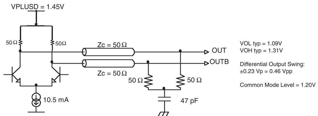
**Figure 13-10.** Unterminated Differential Outputs (Optional)
