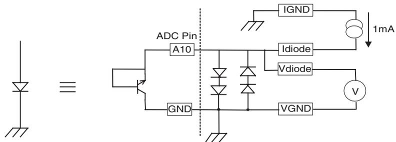
**13.7.7 Junction Temperature Diode Transfer Function**
