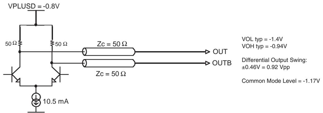
**13.6.2 LVDS Differential Output Loading Configurations**
