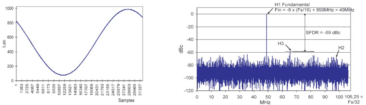
Figure 10-16.  $F_s = 1.7$  Gps and  $F_{in} = 1699$  MHz, -1 dBFS; Decimation Factor = 8, 32 kpoints FFT
