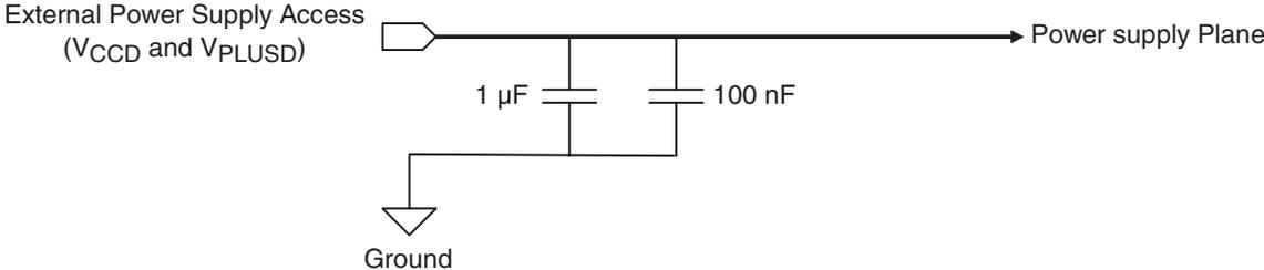
Each group of neighboring power supply pins attributed to the same value should be bypassed with at least one pair of 100 pF in parallel to 10 nF capacitors. These capacitors should be placed as close as possible to the power supply package pins.
