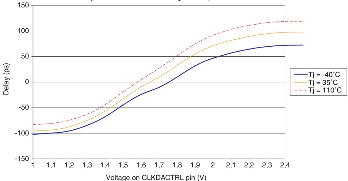
The tuning range is varying linearly over the specified temperature range. The longest tuning range is obtained at hot temperature.
