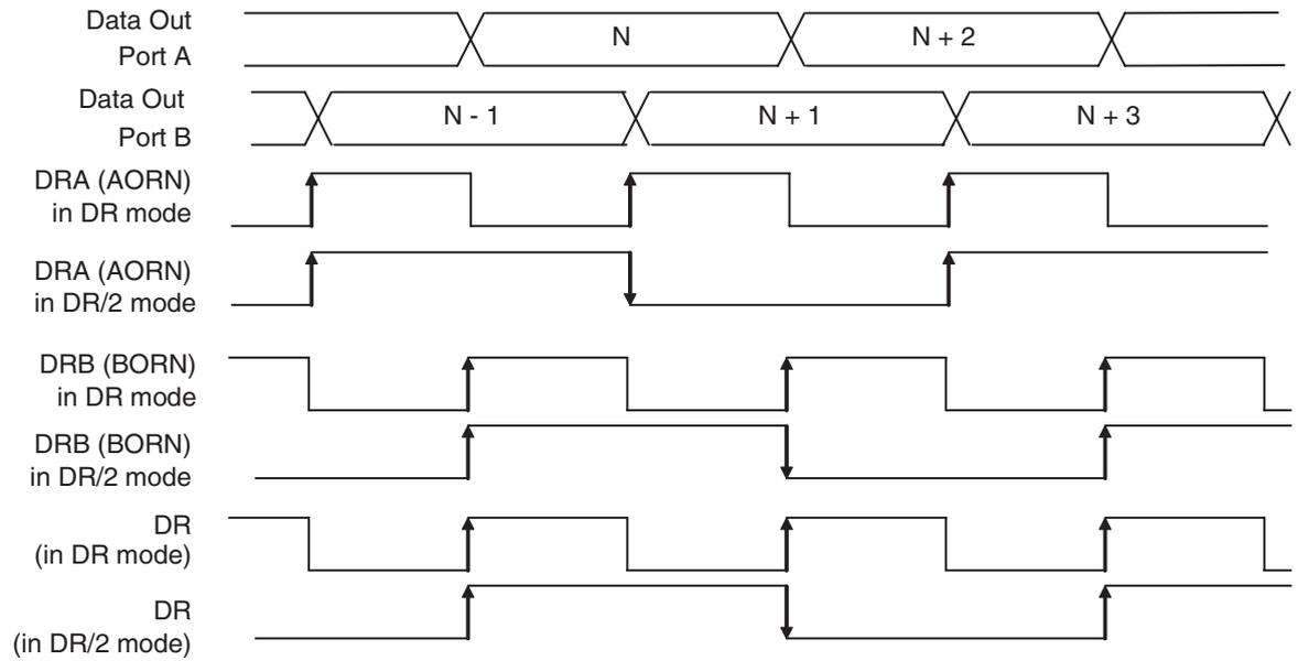
Figure 5-7. Staggered Mode in 1:4 Ratio (STAGG = 0)
