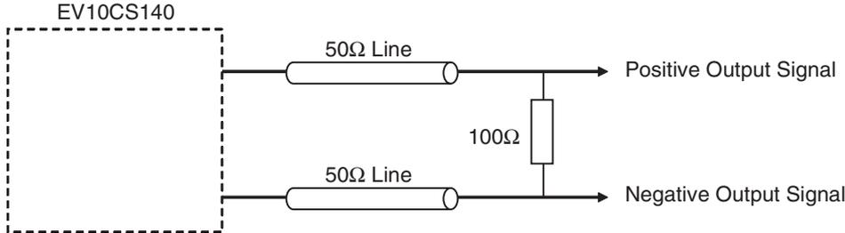
Note: in 1:2 DMUX Ratio, the unused outputs of Port C and D can be left floating. Refer to [Section 5.5 "Programmable DMUX Ratio"](#) on page 14.
