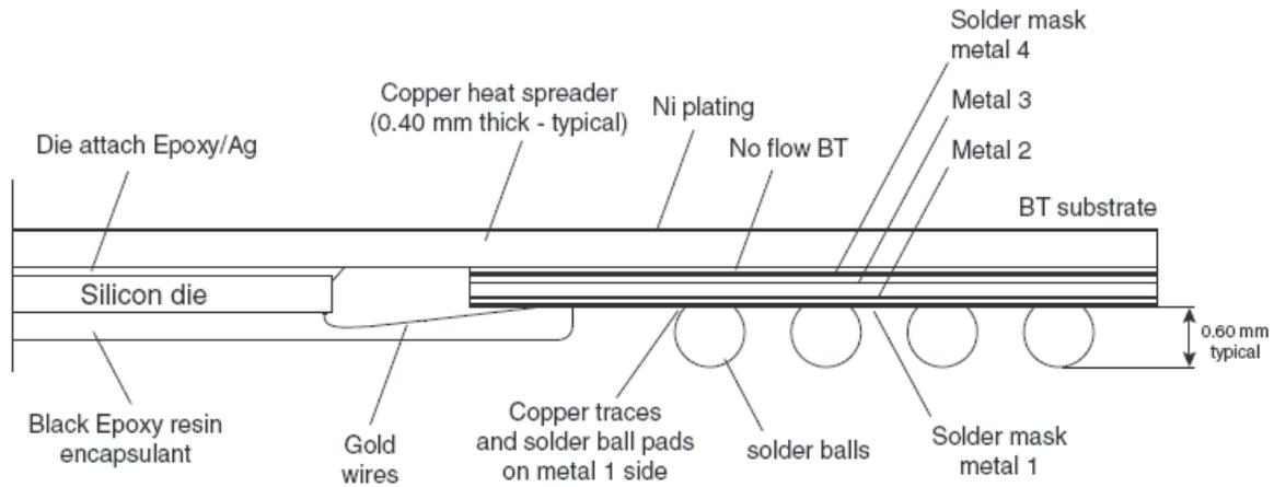
Note: In the DMUX package (see above), the die's underside is attached to the copper heat spreader so the copper heat spreader is at GND (0V). It is recommended to electrically isolate the copper heat spreader from the heat sink if a heat sink is used, in which case adequate low Rth electrical isolation should be used.
