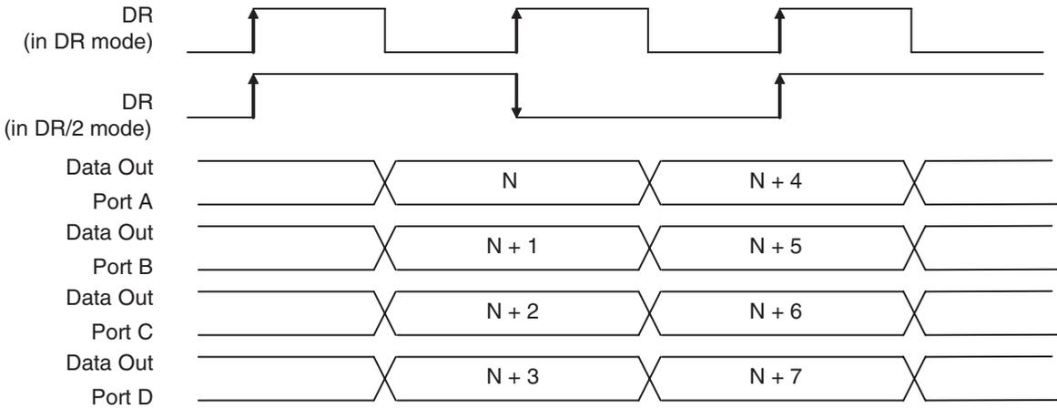
**Figure 5-6.** Staggered Mode in 1:2 ratio (STAGG = 0)
