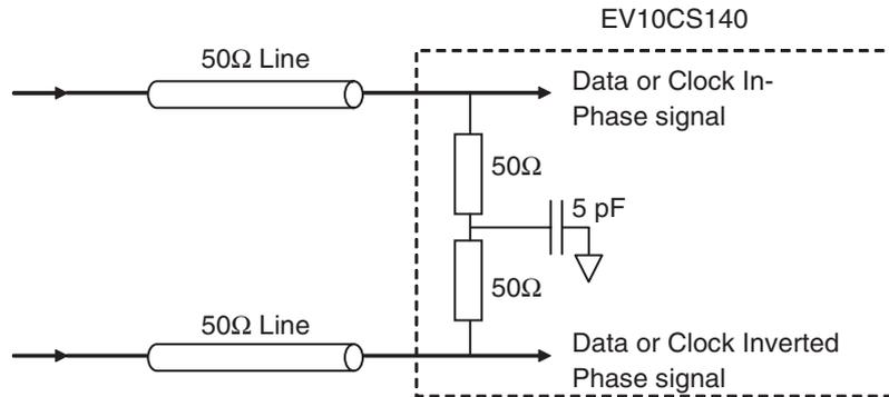
The input clock has to be used in CLK/2 mode (active on rising and falling edge).
