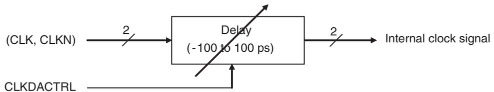
**Figure 5-9.** CLKDACTRL Transfer Characteristics of the Delay Cell
