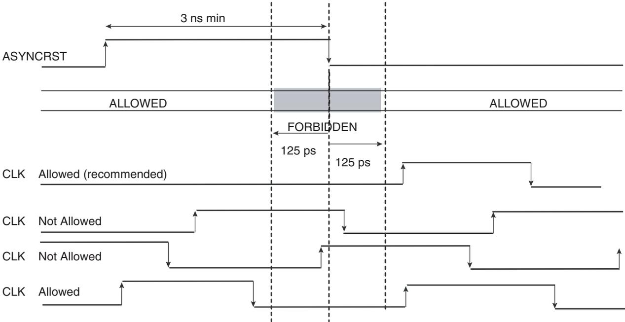
It is highly recommended to stop the clock at the Low level when ASYNCRST is active (high level). Note that when e2v’s ADCs are in reset, the ADC Data Ready output (input clock of the DMUX) is stopped at the low level. In the case where the clock can not be stopped during the reset (note recommended), it is not allowed to have an active edge (rising and falling edge) of the CLK clock within a ±125 ps area around the falling edge of ASYNCRST.
