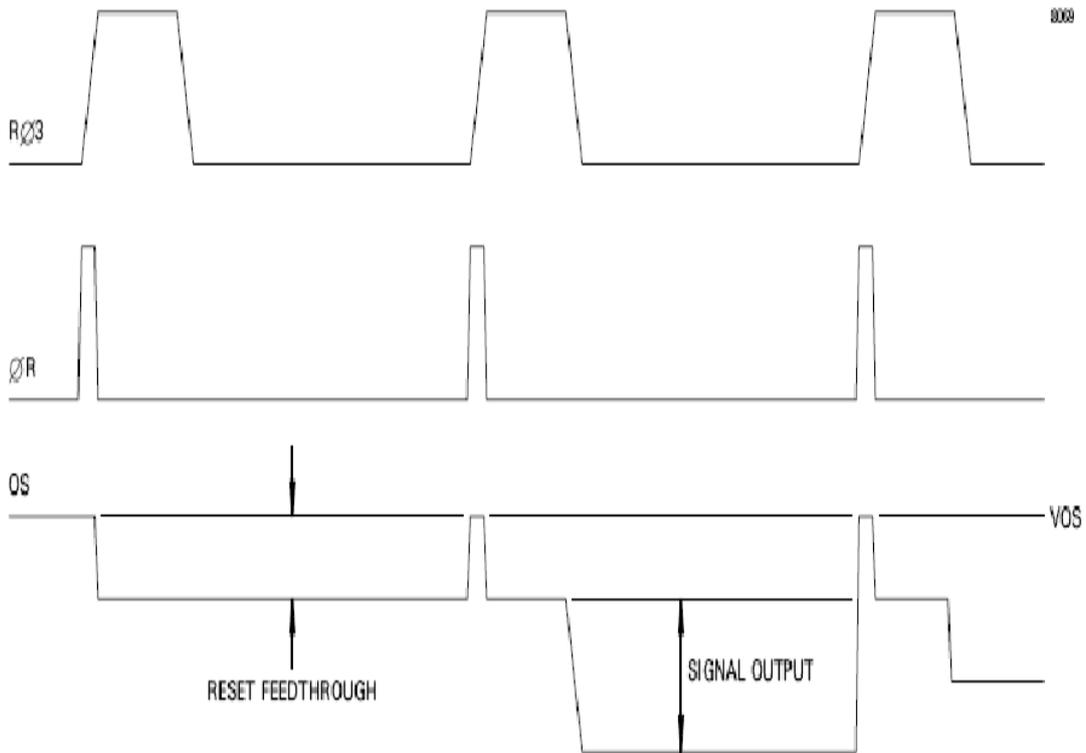
**Figure 9: EXAMPLE FRAME TIMING DIAGRAM**
