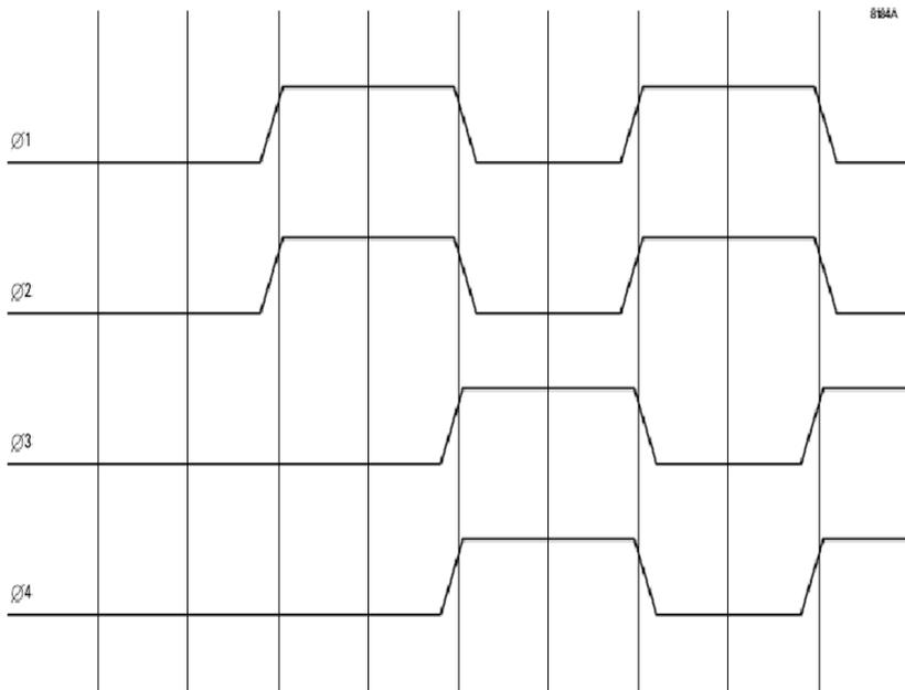
**Figure 5: CLOCKING SCHEME FOR MULTIPLICATION GAIN (sinusoidal RØ2HV pulse)**
